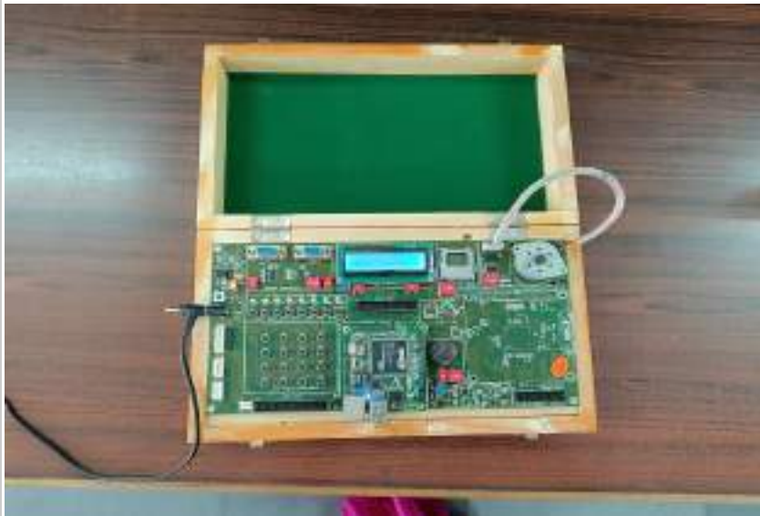
Figure B.5.8.2. STK-9302 trainer for ARM9 Controller
